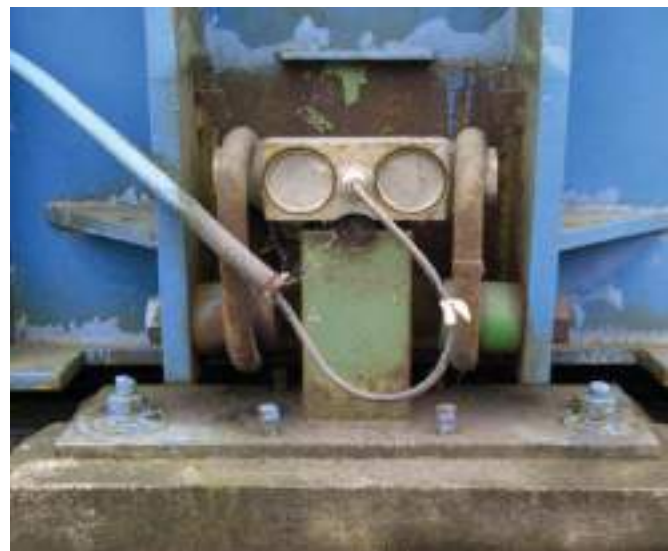
Double-ended shear beam load cells are supported in the center and linked to the weighbridge on each end.
