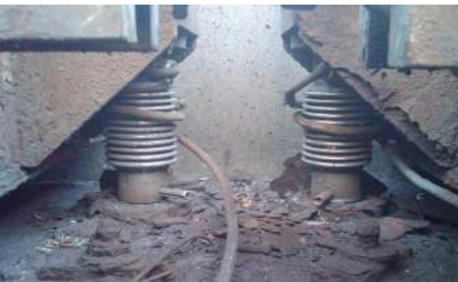
If a compression-style load cell has inadequate anti-rotation features, eventually the cable can wrap around the load cell and break.
