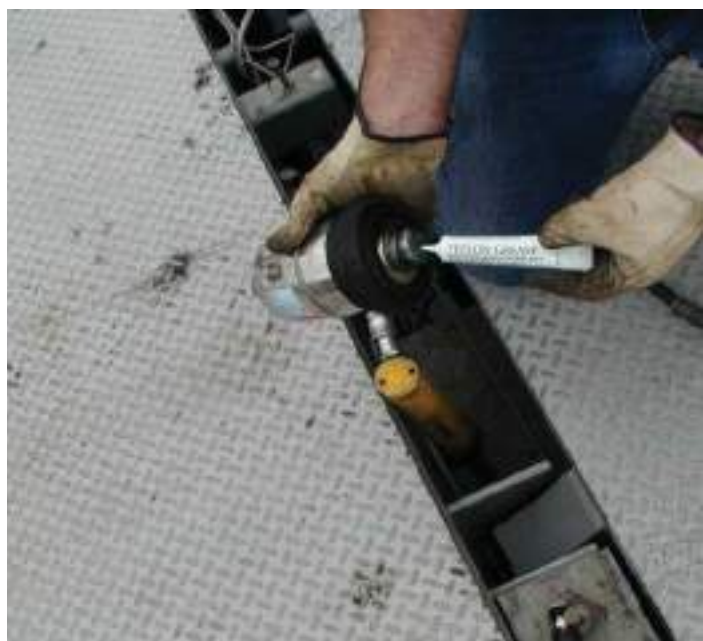
Some areas, such as load cell mating surfaces, require periodic lubrication
