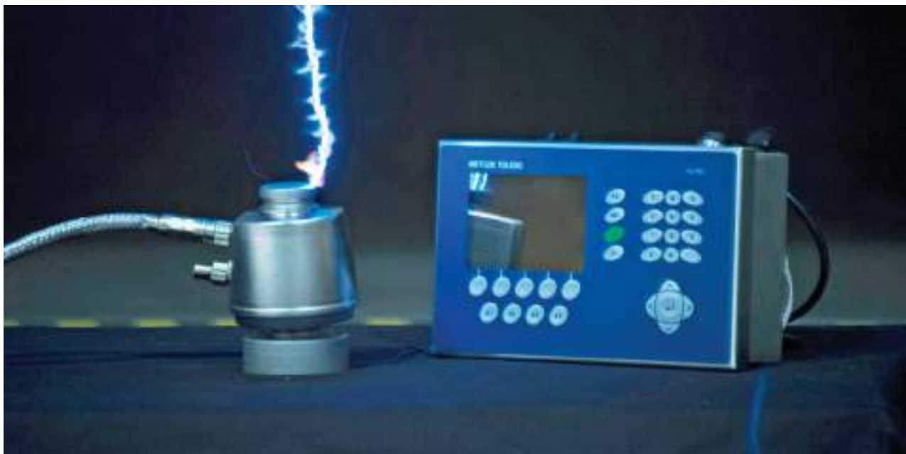
A POWERCELL® PDX® load cell connected to an IND780 terminal during a lightning test
