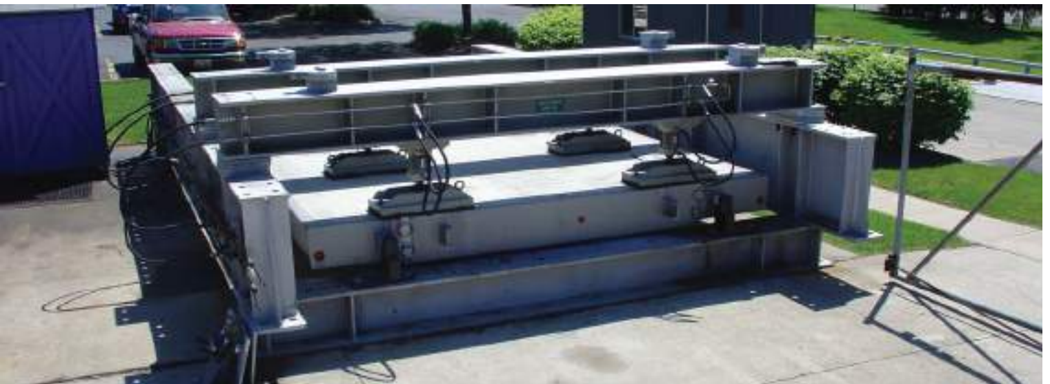
The weighbridge module lifecycle testing machine used by METTLER TOLEDO replicates the forces of trucks driving over the scale.
