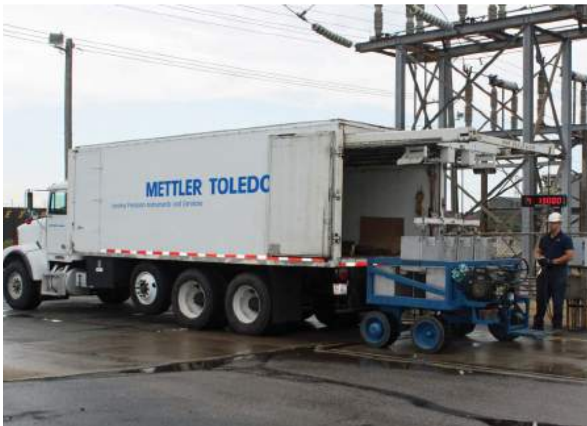
A calibration check can be performed with large test weights that are loaded onto a motorized cart. The technician moves the cart to various points on the scale with different amounts of weight to test for consistent accuracy from the scale
