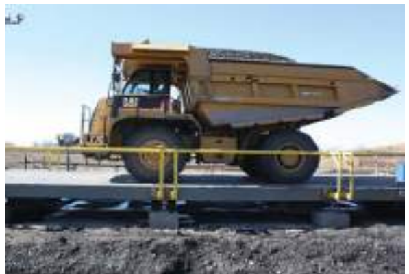
An open-sided scale design can aid in serviceability
