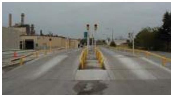
Scale-mounted guiderails are attached to the side of the weighbridge modules with bolts or welded brackets
