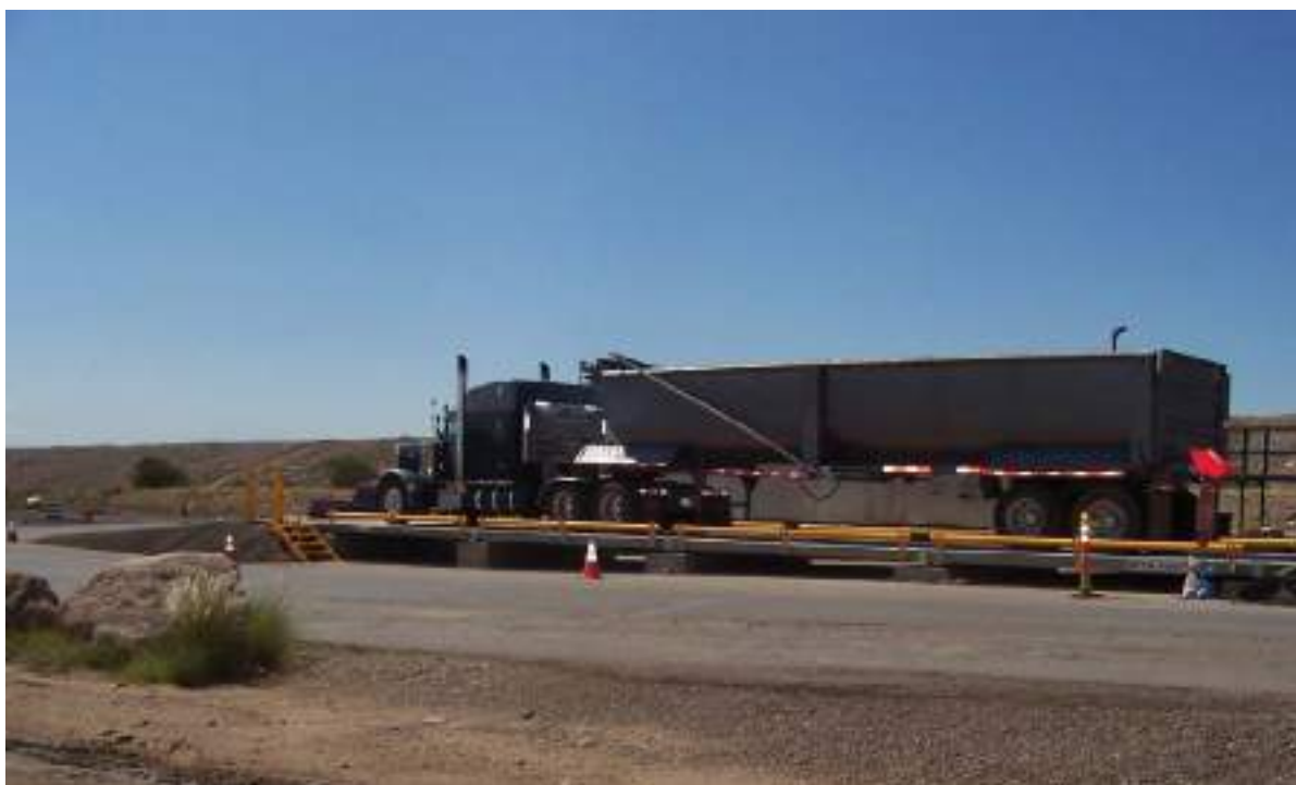
Keeping the scale area clean helps prevent weighing errors caused by debris
