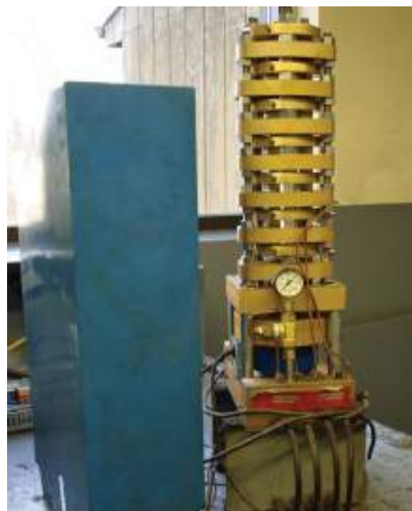
The hydraulic load cells are each connected to the large totalizer unit
