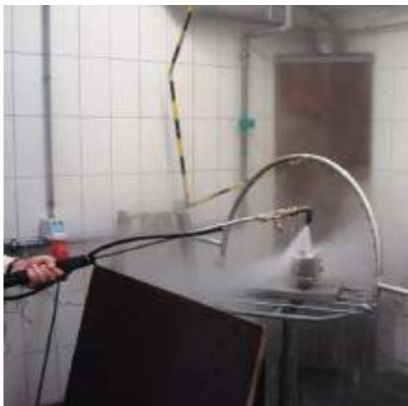
A POWERCELL® PDX® load cell undergoing an IP69K test with pressurized spray
