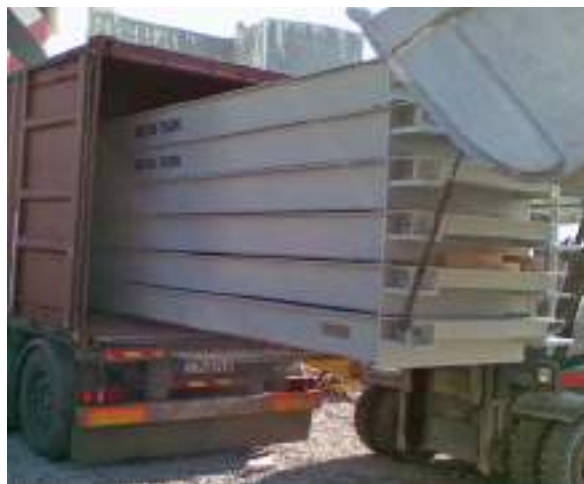
Some manufacturers can offer containerized scales to simplify transporting the scale long distances, or to remote areas
