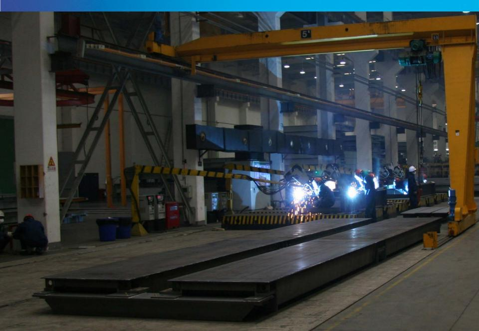
Modules exiting blasting machine- Steel shot blasted 6 sides
