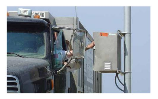
Unattended weighing is an effective strategy for increasing productivity and reducing operating costs. It introduces self-service efficiency to a vehicle-weighing operation. An unattended solution is ideal for scales in remote locations, scales that operate around the clock, and facilities with multiple scales.
