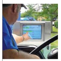
Unattended terminals allow drivers to enter data with a keyboard, touch screen, or badge reader (AWID, SmartPass, bar code, magnetic card, etc.).
