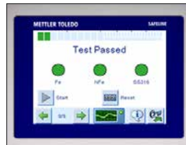
An on screen message confirms the test status for each metal type. The green light indicates a pass.
