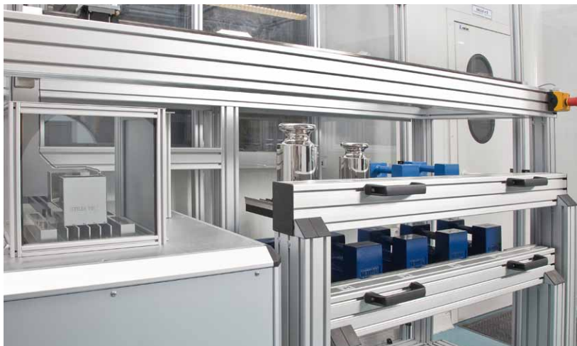
High Load Comparator (AX32004-M10) from METTLER TOLEDO for automatized mass determination of grip handle and knob weights from 1 kg to 20 kg.
